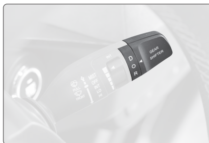
Fig. 29 - Gear selector - Located at the tip of the right-hand lever, behind the wheel.
