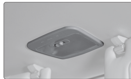
Fig. 107 - Courtesy light on roof.
