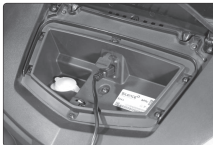
Fig. 120 - Vehicle connection point.
