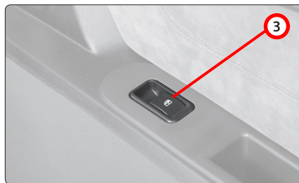
Fig. 109 - Close-up of passenger door: window control.
