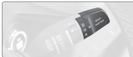
Fig. 31 - Gear selector - Located at the tip of the right-hand lever, behind the wheel.
