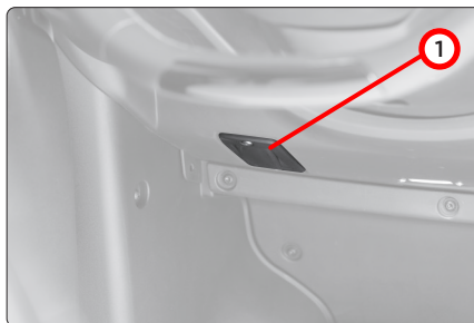
Fig. 106 - Lever to open front bonnet.
