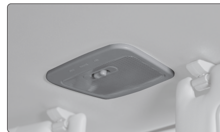
Fig. 115 - Courtesy light on roof.
