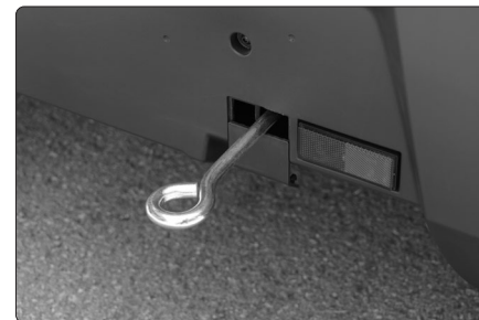
Fig. 16 - Placement of ring on the rear part.
