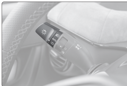
Fig. 110 - Light control - Located to the left of the wheel.
