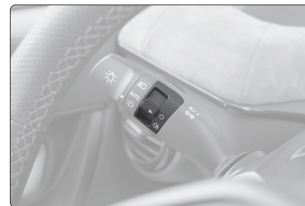
Fig. 111 - Light control - Located to the left of the wheel.
