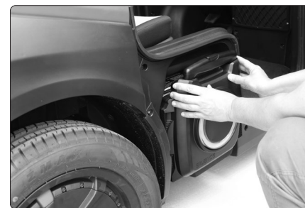
Fig. 137 - Inserting the battery.
