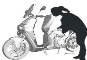
Press de latch. Remove the battery pack.
