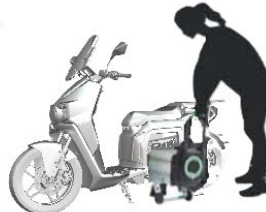
Transport and insert the battery pack into the scooter.
